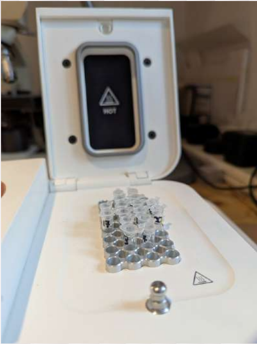
PCR tubes loaded into the Bento Lab thermocycler
