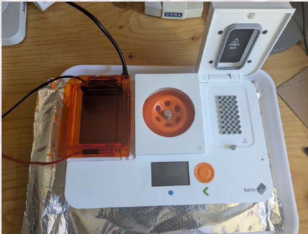
The Bento Lab with the gel tray on the left, mini centrifuge in the middle and the thermocycler for the PCR process in the middle
