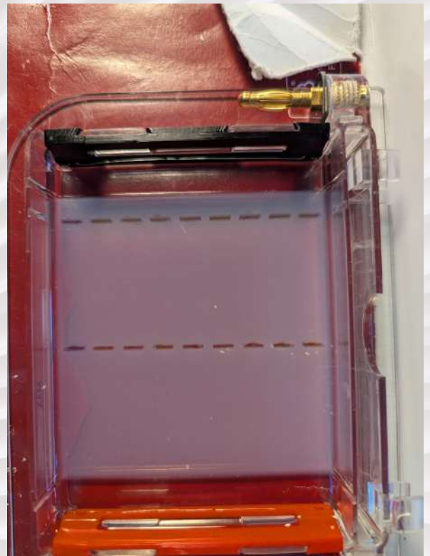
The gel tray ready for adding 3 \mu l of PCR sample into each slot
