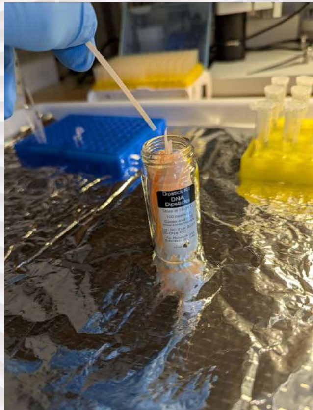
A dipstick to transfer DNA to the PCR mix
